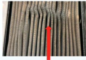
Damage from Backfire
